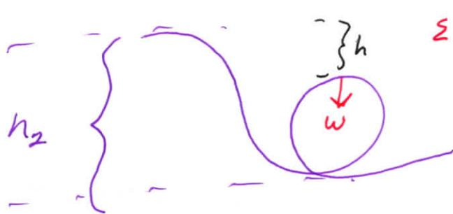
$$\begin{aligned}\sum F_y &= -w = ma_c \\ mg &= \frac{mv^2}{r} \\ g &= \frac{v^2}{r} \\ gr &= v^2\end{aligned}$$
