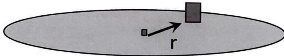
$$\begin{aligned} \sum F_y &= N - w = 0 \\ N &= w \\ N &= mg \end{aligned}$$
