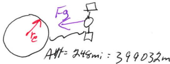
$$r = r_e + Alt = \\ 6.38 \times 10^6 \text{ m} + 399032 \text{ m} = \underline{\underline{6.779 \times 10^6 \text{ m}}}$$
