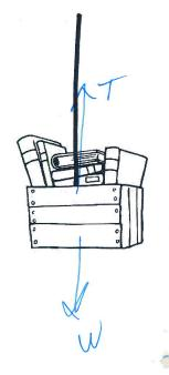
E Fy = T - W = Ma T - W = O (const. Spreed) T = mg : (12Kg/9.8m/s): T = 117.6 W
