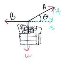
5) The crane pictured below is lifting the 45 kg box, accelerating from rest to 2 m/s in a time of 1.2 seconds. Determine the tension in the cable.
