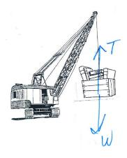
$\sum_{y} = T - w = mq$   $T = m\alpha + mq$   $T = m (\alpha + q)$   $T = m(\frac{v}{z} + q)$   $T = (45/4)(\frac{2mg}{1.25} + 9.8 \frac{mg}{s})$
