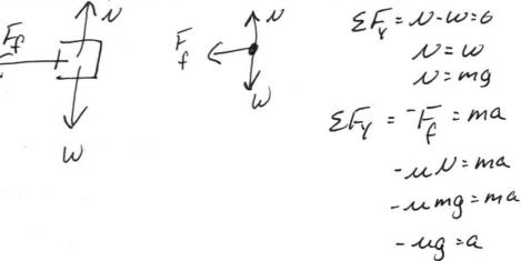
4) A box is riding along in the cargo area of your vehicle. Determine the minimum coefficient of friction between the box and the "floor" of the cargo area so the box doesn't slide when the vehicle accelerates at rates as high as 4m/s2.
