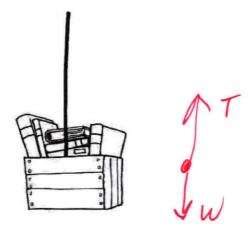
$\Sigma F_{Y} = T - \omega = ma$  T = ma + mg T = m(a + g) T = (2kg)(3m/s + 9.8m)T = 25.60
